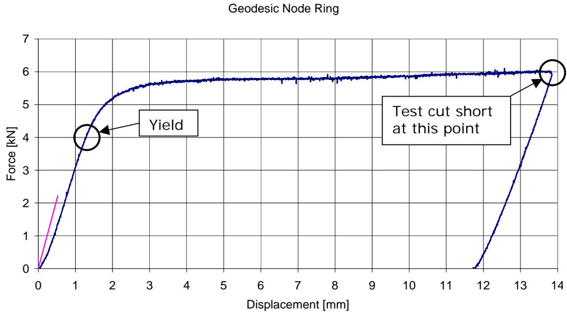
**Figure 8: Node ring force - deflection curve**
