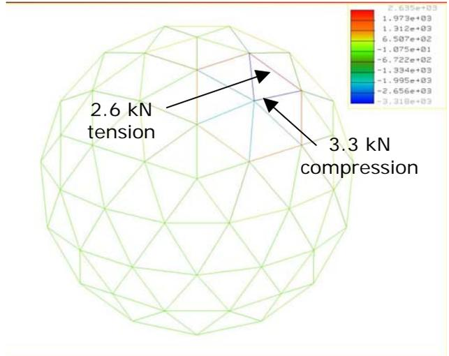
**Figure 17: 4,000 N suspended from node 5**
