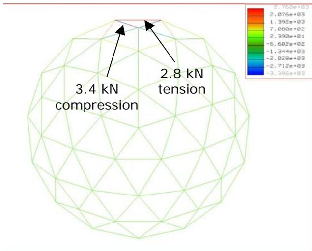
**Figure 18: 4,000 N suspended from node 7**
