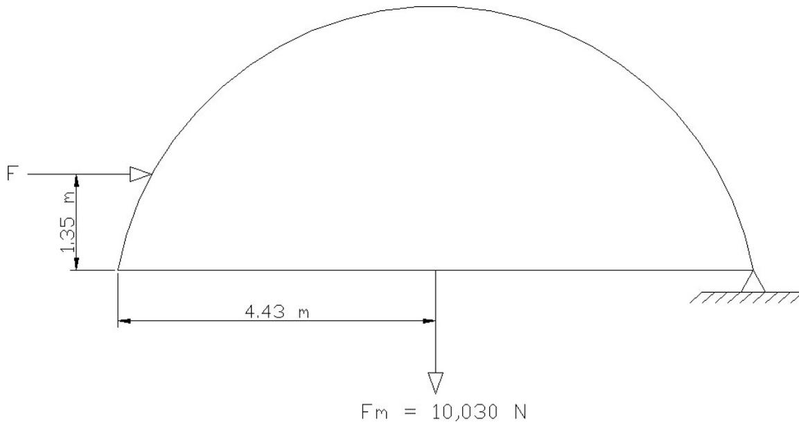
The wind velocity required to create a force of this magnitude is approximately 100 m/s which is well below the 30 to 40 m/s wind speeds used in region A wind calculations so overturning should not be a problem with this structure in region A winds.
