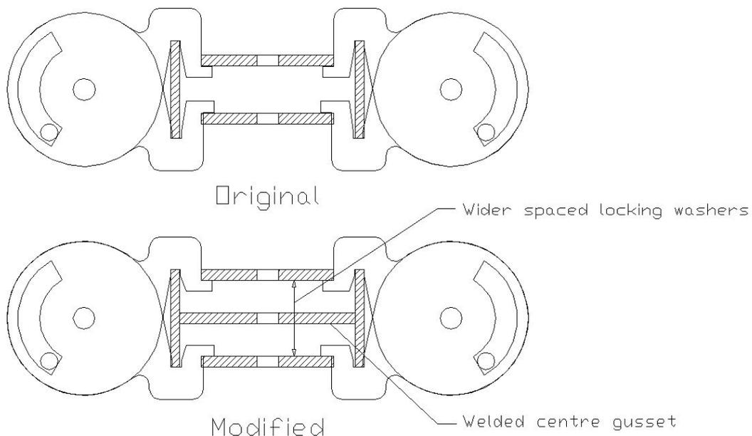
**Figure 20: Differences between original and modified nodes**
