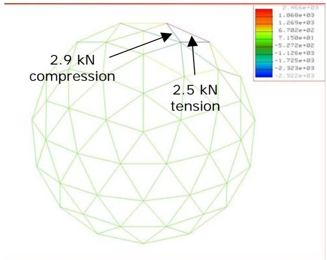
**Figure 19: 4,000 N suspended from node 8**
