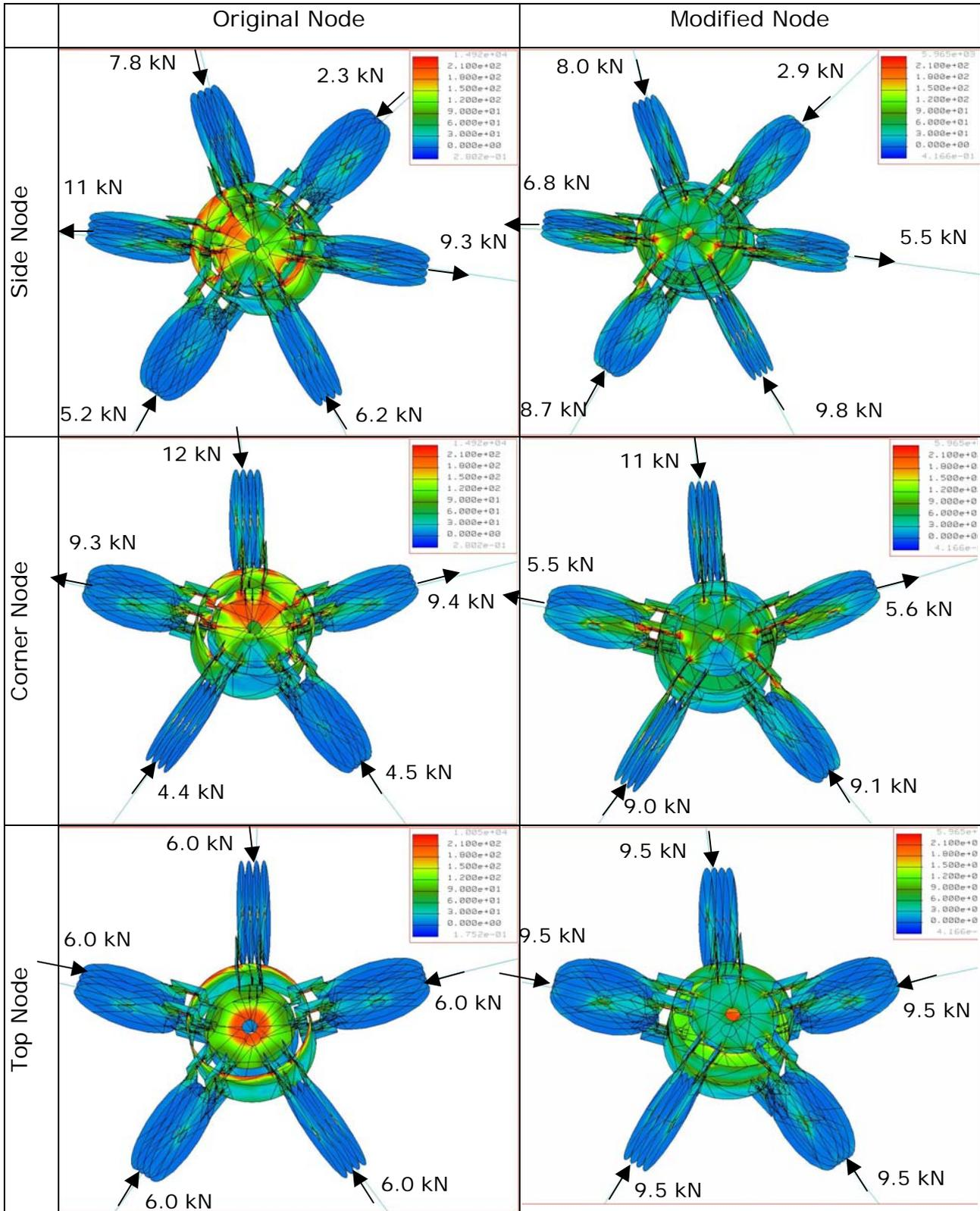
Figure 21: Comparison between strength of original and modified nodes
