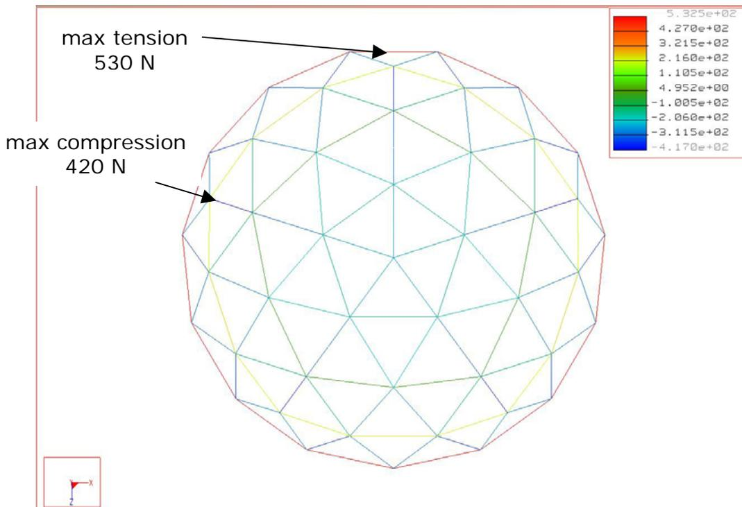
**Figure 12: Beam forces due to structure dead weight**
