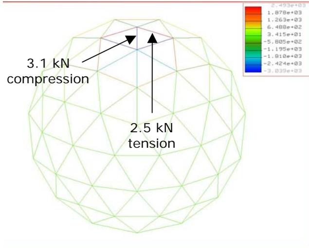
**Figure 16: 4,000 N suspended from node 4**
