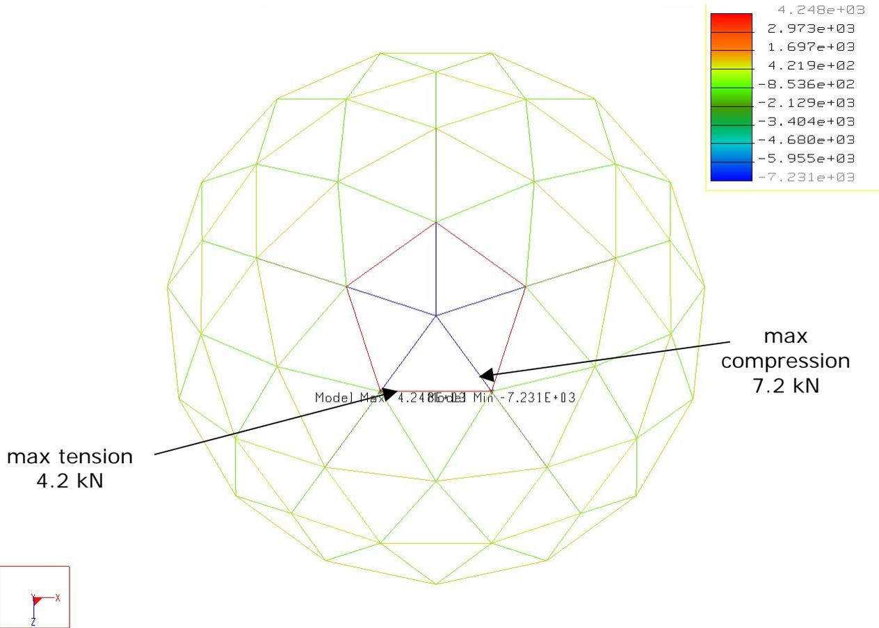
Figure 23: 6,000 N suspended from centre node (worst case single node loading)
