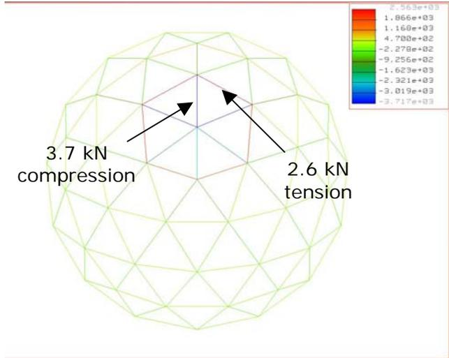
**Figure 15: 4000 N suspended from node 2**
