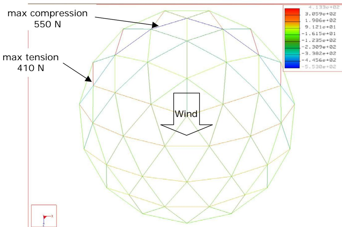
**Figure 10: Beam forces under serviceability limit state**
