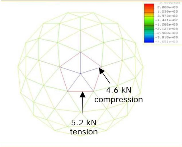
**Figure 14: 4,000 N suspended from node 1**
