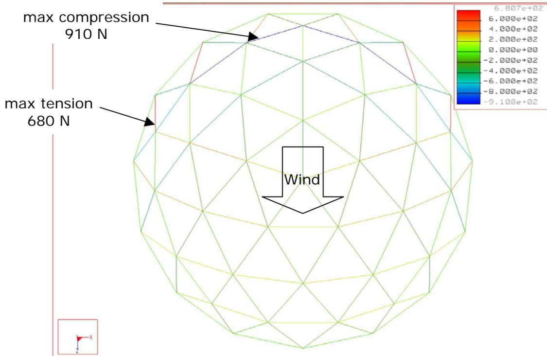
**Figure 11: Beam forces under ultimate limit state**
