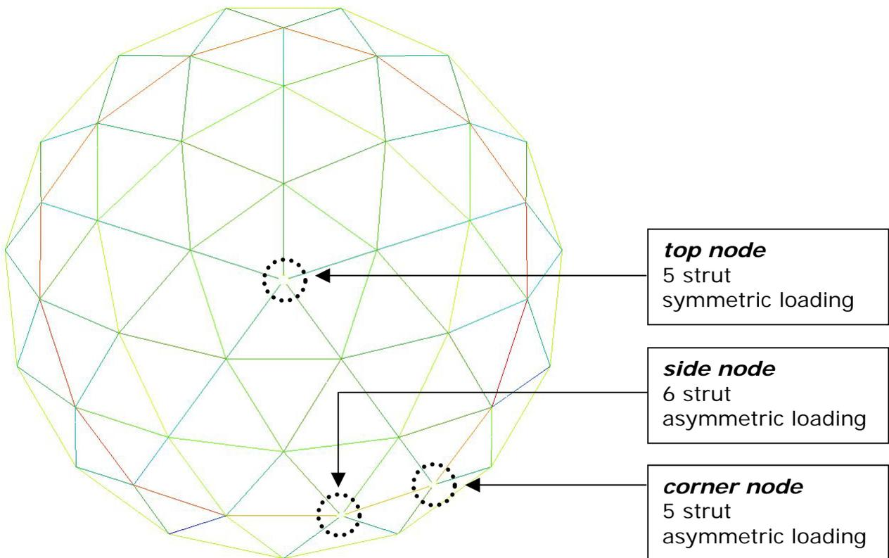
**Figure 6: Location of nodes analysed on the structure**
