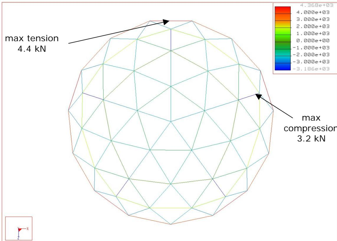
**Figure 13: 2,000 N suspended from all nodes**
