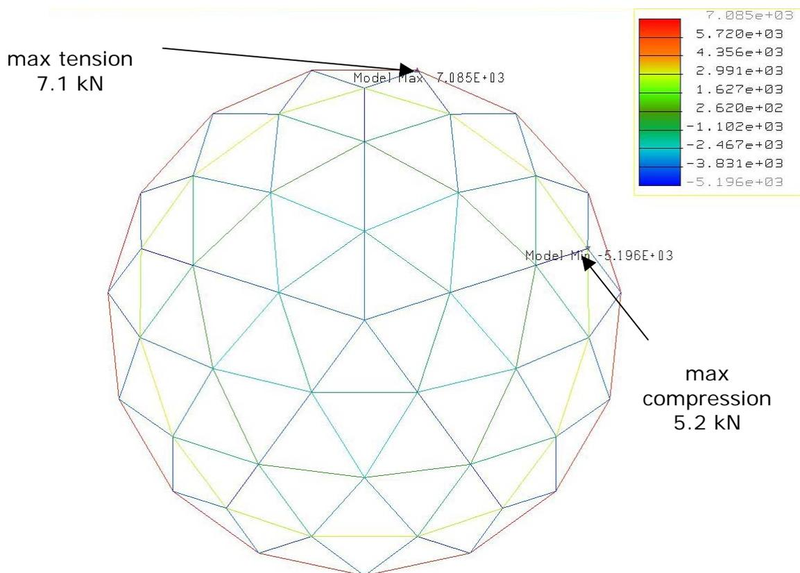
**Figure 22: 3,000 N suspended from all nodes**
