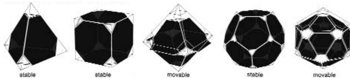
2.5 Platonic polyhedra as bar and node or pure plate structures (a) tetrahedron, (b) cube or hexahedron, (c) octahedron, (d) dodecahedron and (e) icosahedron. (Diagram courtesy: Ture Wester)
