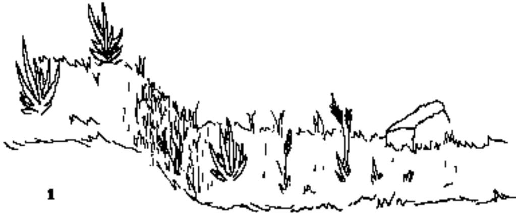
Clear all obstructions, debris and organic material, such as trees, bushes and grass, off the ground on which the EcoShell will be built.
