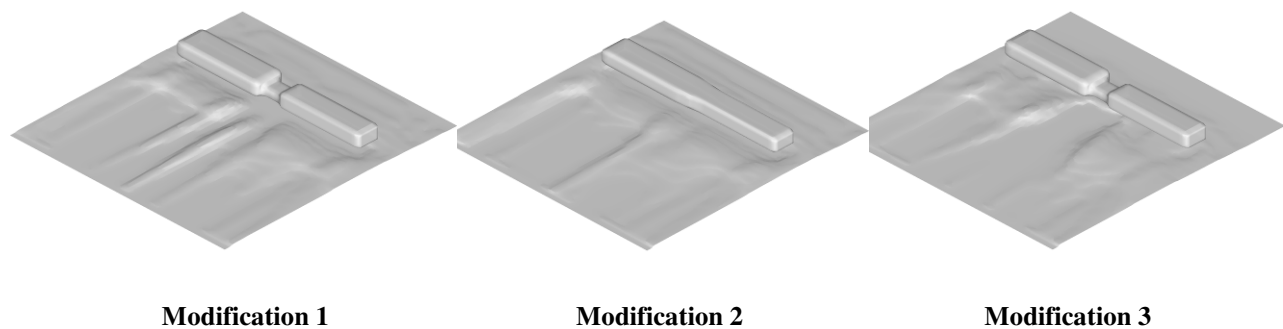
Figure 10: Three-dimensional snow drift predictions for three mitigation concepts
